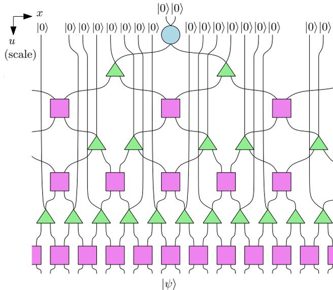
**Figure 2:** MERA as a quantum circuit.
