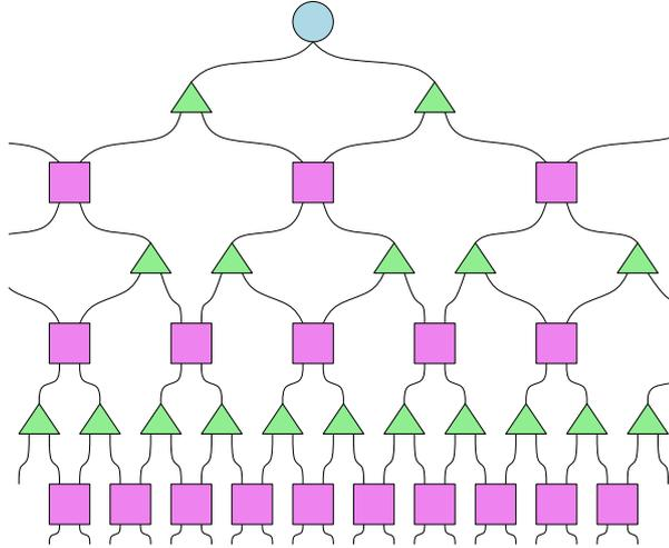
**Figure 1:** A MERA tensor network. Isometries are shown as green triangles, and disentanglers as violet squares.
